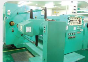
2-2 UN- Winder (Machine that unravels film)
