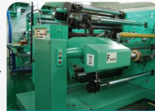
2-3 RE-Winder (Machine that rewinds the film)
