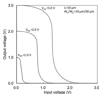
**Fig. 1. CMOS inverter made up of CLC LTPS TFTs with HfO<sub>2</sub> gate stack.**
