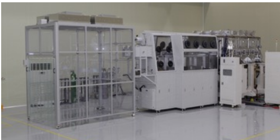
Fig. 1. Sixth generation batch atomic layer deposition system (Lucida™ GD-600)
