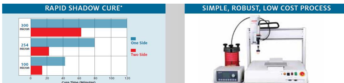
Fig. 1. Primer Shadow Cure Profile and Application
