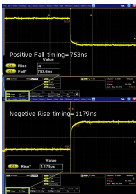
Fig. 8. Before HAVDD Improve
