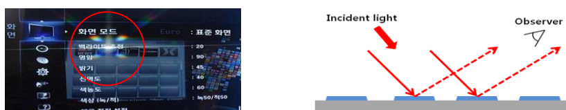
Fig. 1. (a) Iridescent reflection in LCD panel (b) Constructive interference in fine slit pattern
