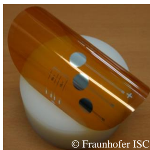
Fig. 1. Flexible polymer substrate with ORMOCER ® thin film transistors.
