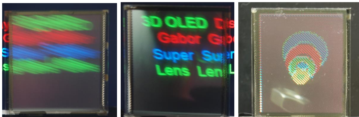
Fig. 1. Transparent OLED display with lenticula destroys the background text (left). The display with Gabor super-lens displays the background image floating in front (middle). Multiview 3D image (color rings) can be superimposed with floating image of the background 3D object (right)
